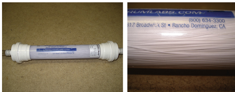
Fig. 2. Phantom used to simulate airways properties in the T_2^* measurements.
